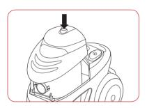
Remove the hose and tubes for the machine. Hold the handle and press the release button.
