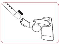
4. Push the telescopic tube into the desired floor tool/accessory until it fits into place. To remove, just separate.
