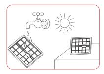
3. Rinse the HEPA Filter in luke warm water and dry completely before replacing into the container.
