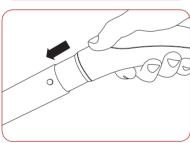
2. Fit handle into the telescopic tube until it clicks into place. To remove, press button and separate.
