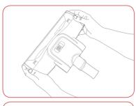
Depress the buttons on both sides of the turbo brush, the plastic cover will release.
