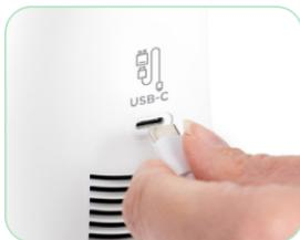
1. Insert the USB charger into the charging port on the back of the vacuum cleaner.
