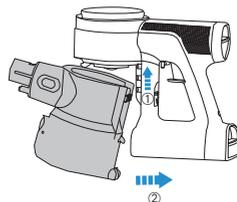
When re-attaching the dustbin, hold on an angle and slot the top of the dustbin into the hook on the main body. Push upwards until the hook is fixed into the slot on the dustbin and then it clicks into place.
