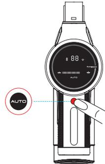
When in Manual mode, press AUTO for 2 seconds until the AUTO indicator illuminates.
